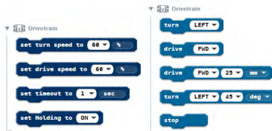
Figure 8. Drivetrain code blocks
